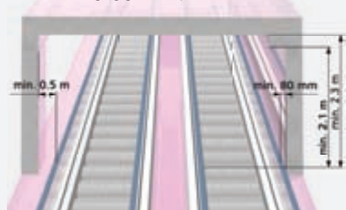
min. 0.5 m, otherwise wedging guard required
